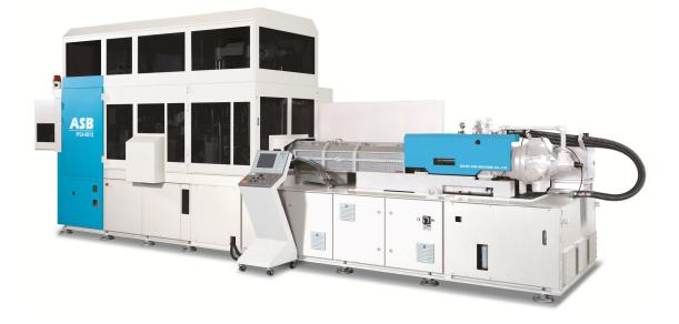
The PF24-8B/12 machine uses ASB's unique and pioneering 1.5-step molding process to injection stretch blow mold PET bottles directly from raw material in an extremely compact space. In order to achieve the same output by alternative molding methods at least 2-3 times the factory floor area would be required.
